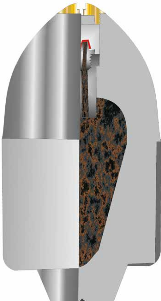
3.73-inch James shell, Type II, sectioned
