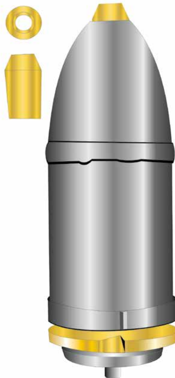
2.94-inch Mullane shell, C. S. brass time fuze adapter
