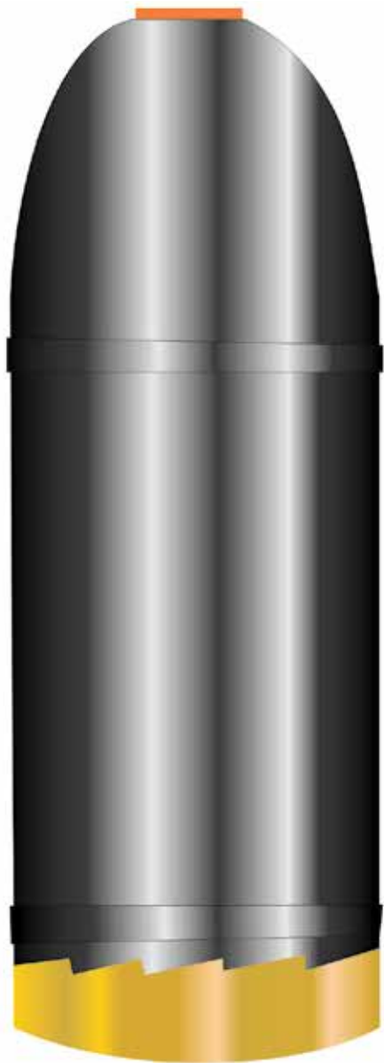
3-inch Brooke shell, time fuze
